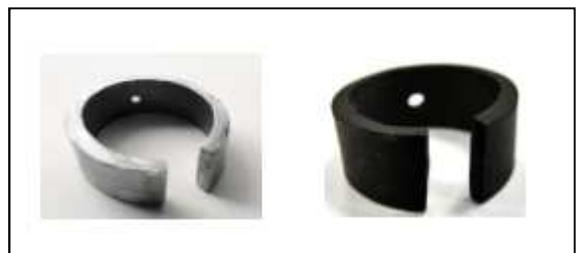
Figure 9. Inconel<sup>®</sup> alloy 600 ring before (left) and after (right) oxidation/lithiation process.
