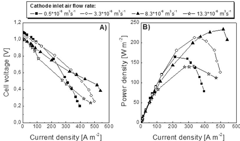
Figure 4. Cell voltage vs. current density (A) and power density vs. current density (B) curves for different cathode inlet air flow rates (fuel: biochar, particle size:  $0.18 \times 10^{-3} - 0.25 \times 10^{-3} \text{ m}$ , electrolyte temperature: 723 K).
