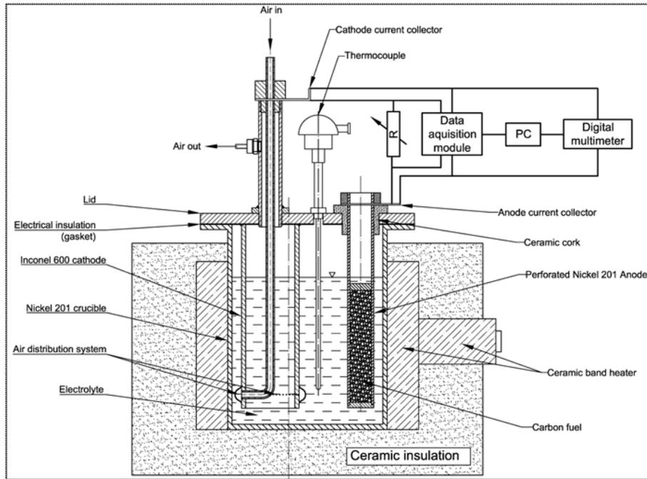
Figure 1. The outline of the experimental DCFC setup.
