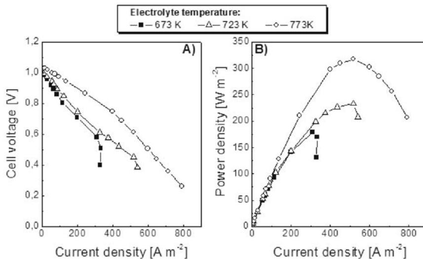
Figure 3. Cell voltage vs. current density (A) and power density vs. current density (B) curves for different electrolyte temperatures (fuel: biochar, air flow rate:  $8.3 \times 10^{-6} \text{ m}^3 \text{ s}^{-1}$ , particle size:  $0.18 \times 10^{-3} - 0.25 \times 10^{-3} \text{ m}$ ).
